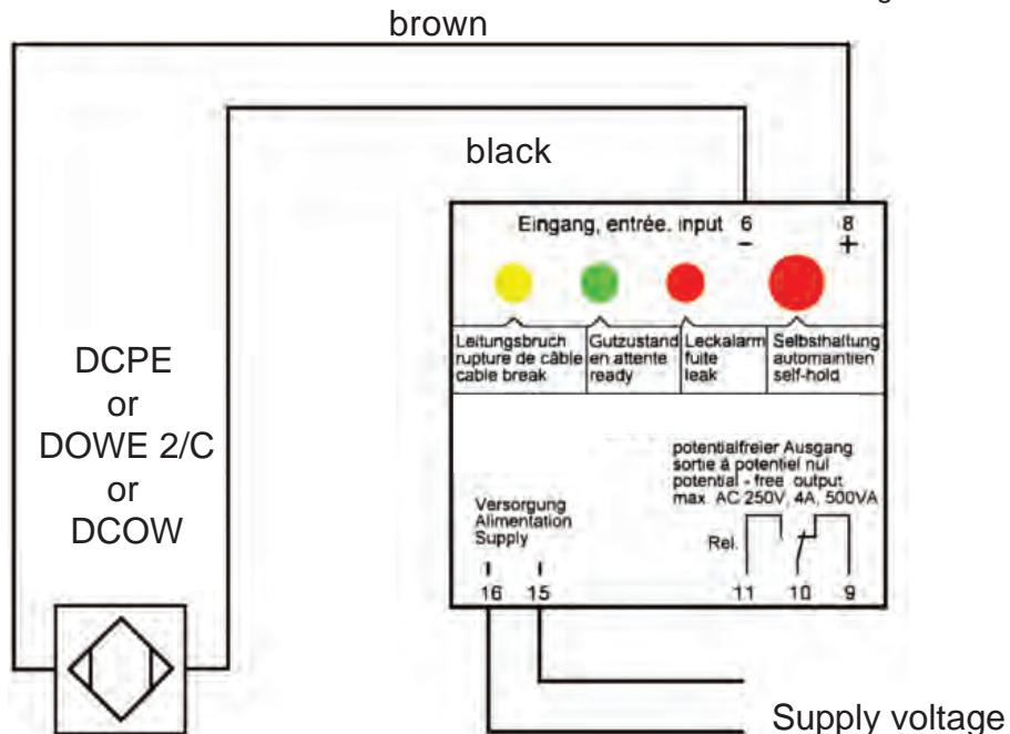
Position of contact when LeakCapacitive 101 without voltage
