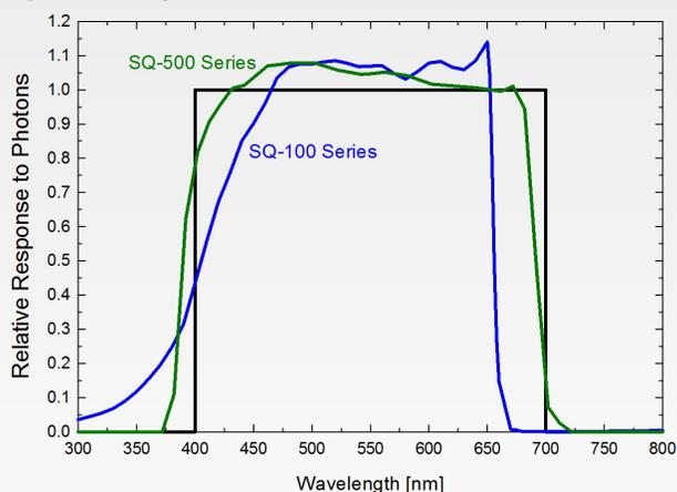
Mean spectral response measurements of six replicate Apogee SQ-100 and SQ-500 series quantum sensors. Spectral response measurements were made at 10 nm increments across a wavelength range of 300 to 800 nm in a monochromator with an attached electric light source. Measured spectral data from each quantum sensor were normalized by the measured spectral response of the monochromator/electric light combination, which was measured with a spectroradiometer.
