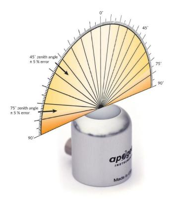
Directional, or cosine, response is defined as the measurement error at a specific angle of radiation incidence. Directional error for Apogee SU-200 series UV-A sensors is approximately ± 2 % and ± 5 % at solar zenith angles of 45° and 75°, respectively.
